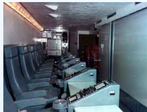
Capsule with 14 crew workstations and movable white boards for status updates and tactical displays
