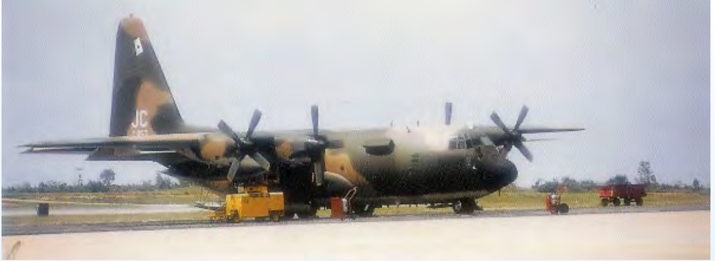
EC-130E based at Korat Air Base Thailand. Note the fuselage mounted air scoops used to cool USC-48 ABCC Capsule
