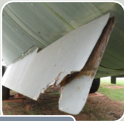
Ventral stabilizer damage due to weather and aggressive lawn maintenance
